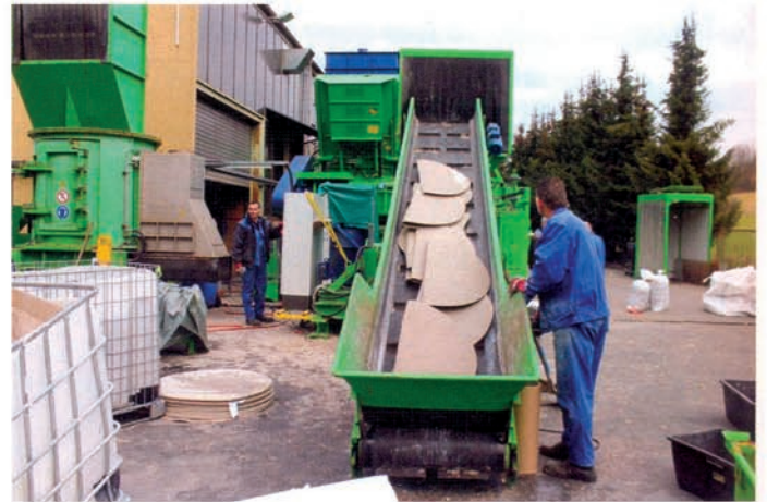
Fig. 2: Feeding cardboard (D-1) as input material
