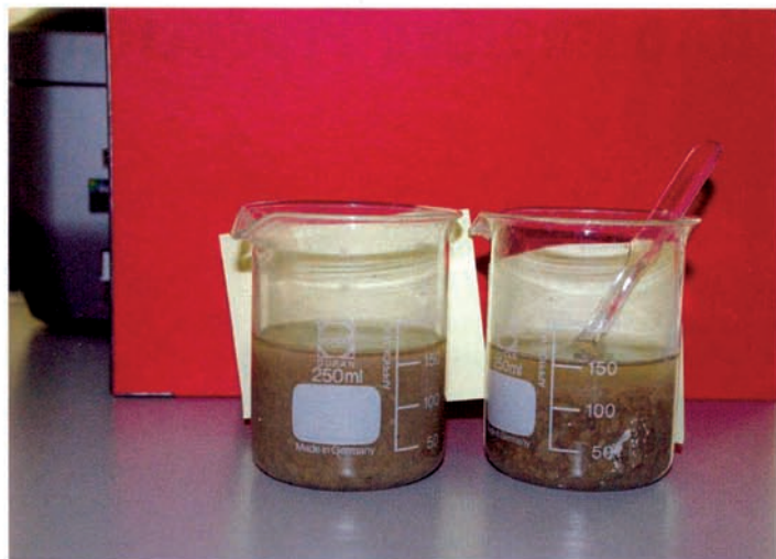
Fig. 5: Fiber stock (D-1); left, after stirring it up; right, after the agitator
