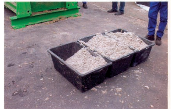
Fig. 3: Output - fiber stock made from cardboard (D-1)
